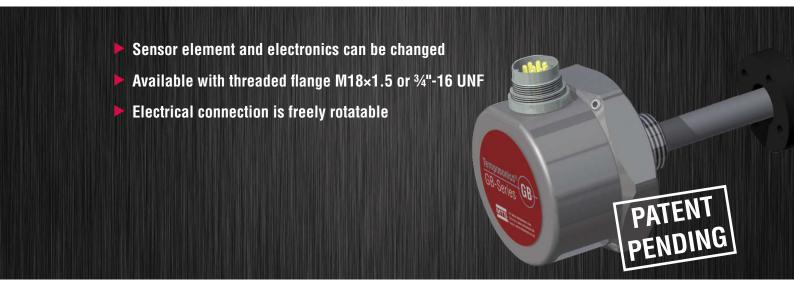
The Temposonics® GB-M / GB-T sensors, designed to be incorporated into hydraulic cylinders, offer many user-adaptable features. The flat and compact sensor electronics housing has an electrical connection that can be rotated 360 degrees to easily achieve the necessary connection orientation. If needed, the sensor element and electronics can be replaced without interrupting the hydraulic circuit – resulting in lower maintenance costs and reduced downtime.
